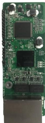
PROFINET communication card EC-TX509
