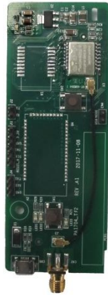
Bluetooth/WIFI communication card EC-TX501/502
