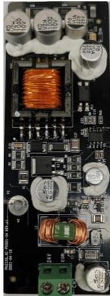
24V power supply card EC-PS501-24
