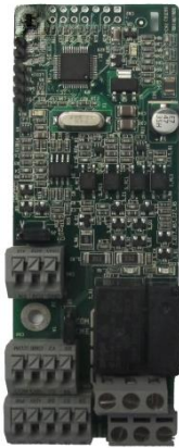
I/O expansion card 1 EC-IO501-00
