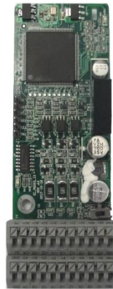
Multifunction incremental PG card EC-PG505-12
