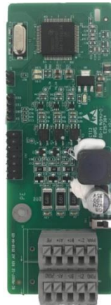
Simplified incremental PG card EC-PG507-12
