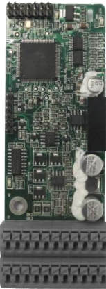
Resolver PG card EC-PG504-00
